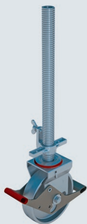
Castor 10.00 kN, Ø 200 mm Installation height: 241 mm plus spindle 500 mm Brake position: 1,000 kg Travel load approx. 400 kg (on level surface)
